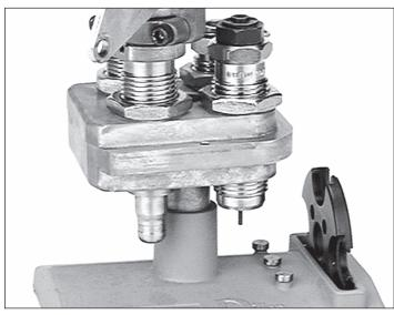
Fig. 15 – A complete, removable toolhead with all of the dies adjusted. Toolhead stand optional.
