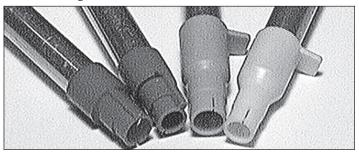
(Repeat of Fig. 14) – The machine comes with two primer pickup tubes (#20060 large, #20059 small) and two primer magazine tubes (#22031 large, #22030 small). They are color coded for easier identification. See color coding information below. The large ones should be used together and the small ones should be used together.
