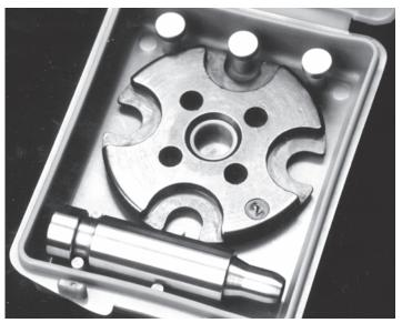
Fig. 4 – This photo shows a complete caliber conversion; the powder funnel, shellplate and locator buttons.
