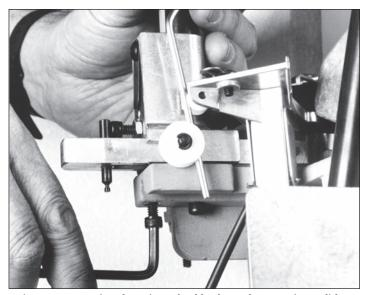
Fig. 13 – Removing the primer feed body to change primer slides. Caution do not over tighten these bolts (#14014).
