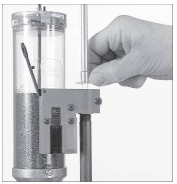
Fig. 26 – Drop the primers into the primer magazine.
