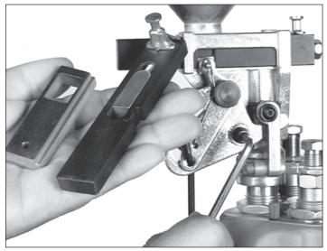
Fig. 24 – After emptying the powder measure, loosen the bellcrank screw (#13904) sufficiently to allow you to remove the powder bar. Insert the new powder bar and reverse this procedure.
