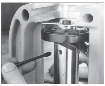
Fig. 10 – Insert the brass-tipped set screw (#13923) and tighten securely.
