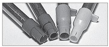
Fig. 14 – The machine comes with two primer pickup tubes (#20060 large, #20059 small) and two primer magazine tubes (#22031 large, #22030 small). They are color coded for easier identification. See page 13 for color coding information. The large ones should be used together and the small ones should be used together.
