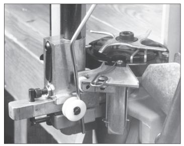
Fig. 11 – This is the proper alignment of the operating rod and the position of the primer slide fully forward with the primer seating cup in the lowered platform.
