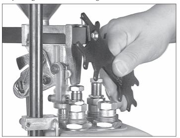
Fig. 23 – Turning the bolt counterclockwise reduces your powder charge, clockwise increases the charge.
