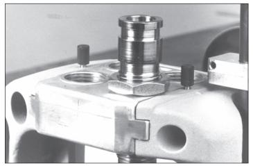
Fig. 17 – This photo shows the powder die in its correct position (Station Two) in the toolhead. The powder die may be higher or lower depending on the caliber it is being adjusted for.
