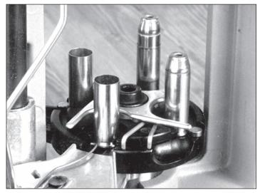
Fig. 16 – A fully loaded shellplate, directly below the proper dies. Clockwise from Station One, the cartridge at this station is resized, deprimed and reprimed. Station Two bells the case mouth (pistol only) and dispenses the powder. Station Three seats the bullet. Station Four crimps the bullet.
