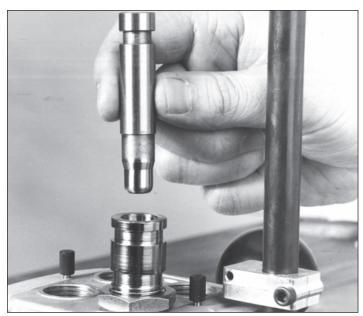
Fig. 18 – Drop the powder funnel into the powder die tapered end first. The funnel should move freely in the die.
