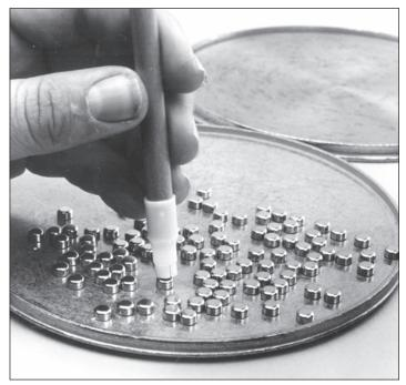
Fig. 25 – Use of the primer pickup tube and the Dillon primer flip tray.
