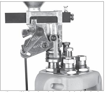
Fig. 20 – This photo shows the large powder bar in its closed position. Note the position of the white bellcrank cube. (Primer system removed for clarity.)
