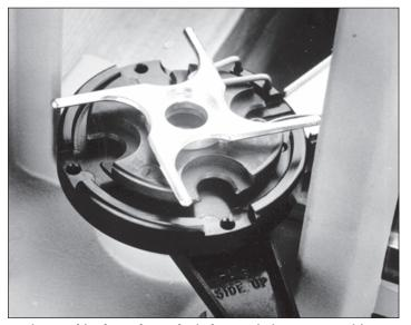
Fig. 7 – This photo shows the index star in its proper position: the locating tabs centered in the shellplate.
