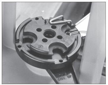
Fig. 6 – Showing the shellplate in its proper position: under the ejector wire with the shellplate number up.
