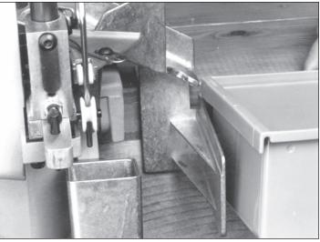
Fig. 3 – The cartridge collection bin (#13839) simply slides onto the bracket and will be in the proper position.
