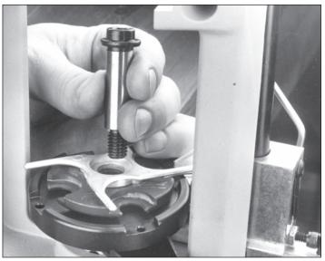
Fig. 8 – Inserting the shellplate bolt, first through the index sprocket then the shellplate.
