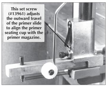
Fig. 12 – The operating rod has moved the primer slide into the primer feed body where it will automatically pick up a primer.
