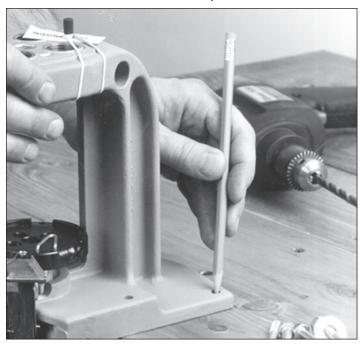
Fig. 1 – Using the machine as a template, mark and drill four 1/4 inch holes allowing 12 inches on each side for your work area.
