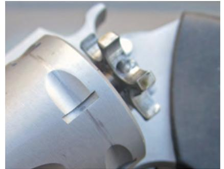
**Top of the page, The Charter .380 Pit Bull, right and left sides. Clockwise from above: When loaded, the rounds are fully recessed. Fully depressed, the ejector clears all the cases. Hard to see, but there in the ejector is one of the little rim-contact parts. Good sights, a wide rear notch and ramp front.**
