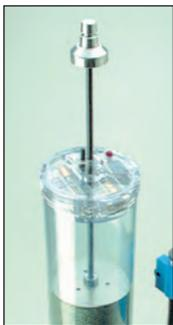
**The Low Powder Sensor** provides an audible and visual reminder when it's time to refill your powder reservoir. When the powder level drops to about 1,000 grains remaining in the reservoir, a buzzer will sound and a bright red LED will light. Designed to fit all Dillon powder measures. Made of clear polycarbonate, it simply replaces the die-cast metal lid supplied with the measure, and operates on two AAA batteries (included).
