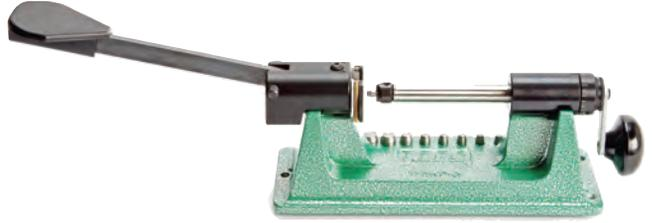
The RCBS Trim Pro-2 manual case trimmer features a spring-loaded "universal" shell holder that will accommodate case head diameters from .250" to .625". Comes with pilot calibers: .22, .24, .25, .27, .28, .30, .35, .44 and .45.
