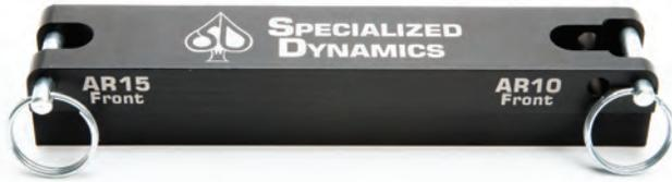
The **Specialized Dynamics AR15/AR10 Armorer's Upper Receiver Block** is made from billet aluminum and holds your upper receiver securely in order to make it easier to install barrels, free-float tubes, muzzle devices, etc. One block fits AR15s and ArmaLite and DPMS platform AR10s.
