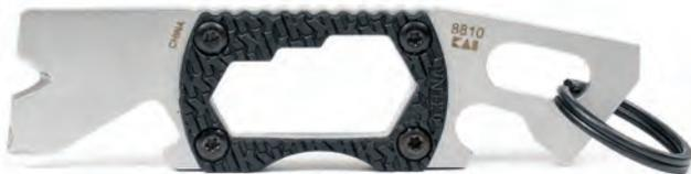
Key chains just got even handier with the new Kershaw PT-2 key chain tool. It offers eight handy functions in a very compact space. The PT-2 (Pry Tool-2) comes in at less than an ounce as well and offers a bottle opener and cap lifter, a pry bar, two screwdriver tips, a wire scraper, and three sizes of hex drives.
