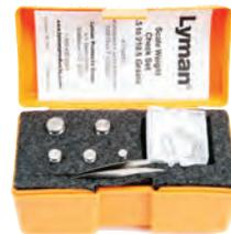
The Lyman Scale Weight Check Set enables you to check/calibrate your scale using known weights. Weight Set .5 - 210.5 Gr.
