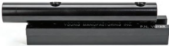
Young Manufacturing's **Upper Receiver Vice** holds any AR15 upper receiver regardless of the manufacturer. Since it supports the receiver from the inside, the outside dimensions are of no concern. Made from aircraft-grade 6061 T6 aluminum and anodized to MIL-A-8625 Type 3 Class 2.
