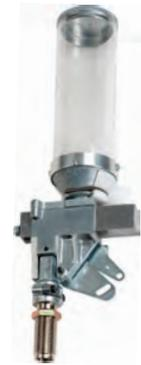
**Dillon's "Belted Magnum" Powder System** features a maximum-capacity steel powder bar that can dispense more than 100 grains of extruded IMR powder. Magnum rifle cartridges can require from 70 grains to well in excess of 100 grains for a single charge. We tested this system with various extruded rifle powders and found that powder charge variations stayed within plus-or-minus three-tenths of a grain.
