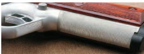
Above: The frontstrap and underside of the trigger guard are checkered 30 lines per inch.
