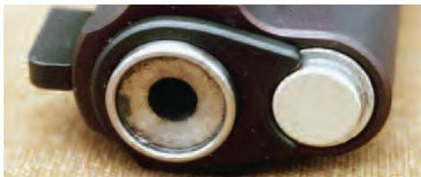
The barrel crown is deeply recessed to protect from accuracy destroying damage.
