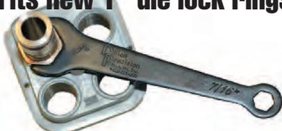
A characteristic of virtually all progressive reloading machines, regardless of brand, is that the dies are set rather close together. When you are first setting up a "naked" machine, there is plenty of wrench room, but if you have a need to adjust a die afterward, it often requires a delicate touch to maneuver a lock ring on a crowded toolhead.
