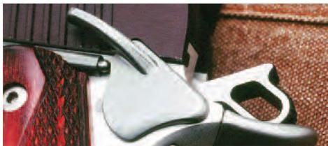
The tab of the extended thumb safety, even when combined with a high-rise beavertail grip safety, does not expose the underlying hole in the frame, a rarity among factory and even most custom 1911s.
