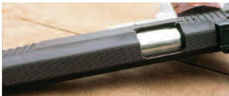
The slide has been flat topped, serrated longitudinally, and fluted on both sides of the serrations.
