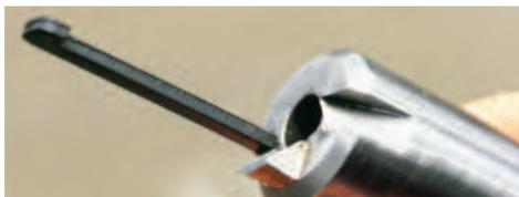
The ejector is a long, hooked piece of metal pinned to the rear of the barrel.
