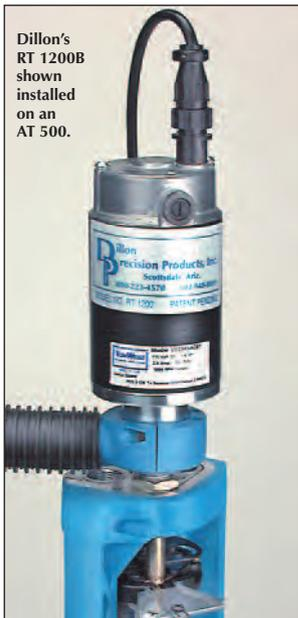
The RT 1200B is used just like a standard size die. The big difference is that while you are pushing the case into the die to size it, a 1/4 horsepower electric motor driving a carbide cutter is trimming the case to length. Chips are drawn off through a vacuum manifold that clamps to the outside of the special size/trim die. (*Vacuum cleaner and hose not included.*) The RT 1200B is equipped with a quick-
