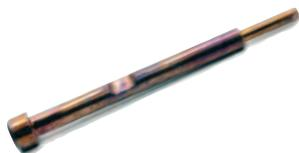
**T**ACCOM's **Enhanced Firing Pin** for Ciener/CMMG .22 Long Rifle AR-15 caliber conversions is a direct-replacement firing pin, made from 17-4 SS heat treated to a condition H900, to present a tough, hard firing pin that won't break or mushroom out after many firings. The tip has been designed to stick out of the hole only .030", so you will not damage your barrel by dry firing your weapon.
