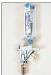
1 i. Powder Measure with Small Powder Bar Installed
