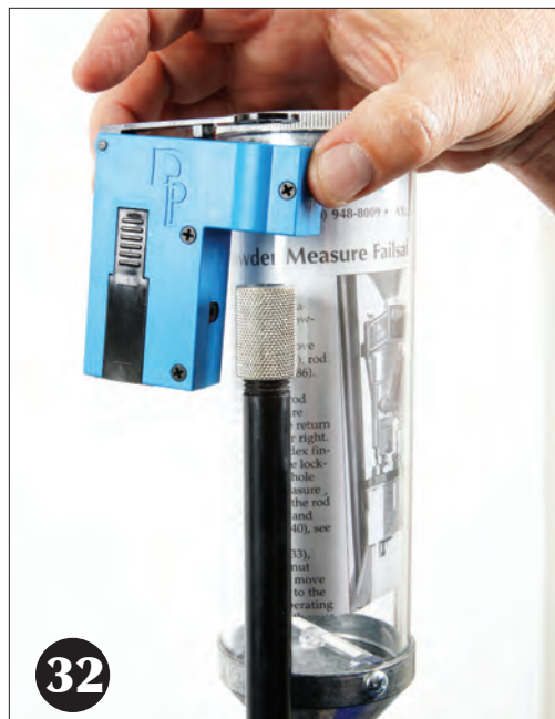
Push the Low Primer Alarm onto the knurled cap at the top of the primer shield as shown in 32 and 33.
