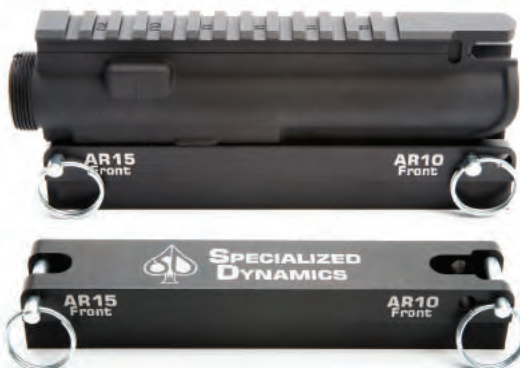
The Specialized Dynamics AR15/AR10 Armorers Upper Receiver Block is made from billet aluminum and holds your upper receiver securely in order to make it easier to install barrels, free-float tubes, muzzle devices, etc. One block fits AR15s and ArmaLite and DPMS platform AR10s. (Sorry, the upper receiver pictured above is NOT included.) O37-43234 $59.99
