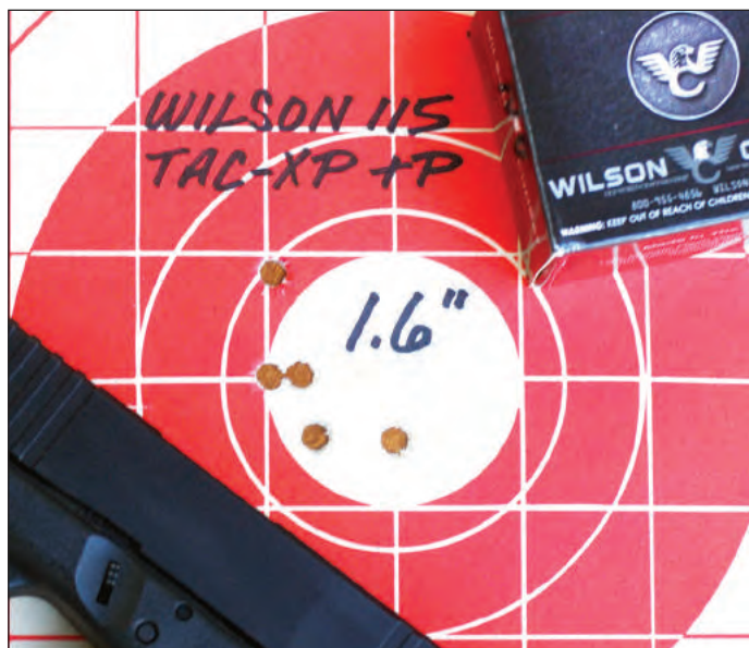
Best accuracy from the Brownells slide/Glock 19 frame hybrid was 1.6" at 50 feet with the Wilson 115-gr. TAC-XP +P.
