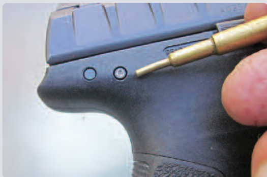
During takedown, you don't pull the trigger. Depressing this little button safely de-cocks the striker.
