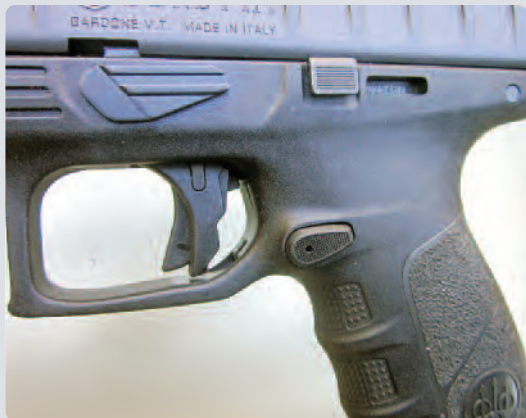
The controls: takedown lever, slide latch, and magazine release.
