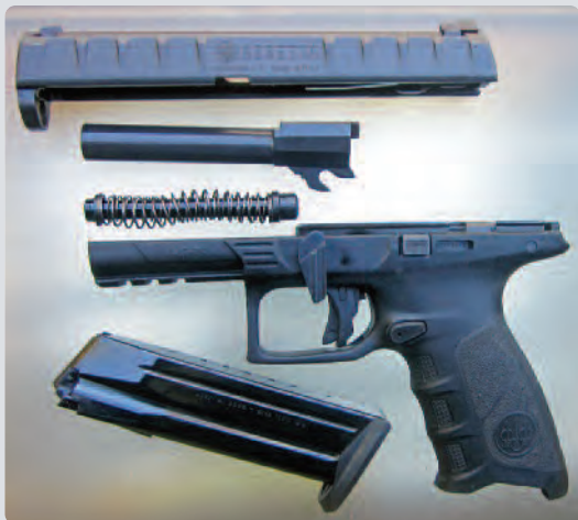
The Beretta APX, fieldstripped. Note the captured recoil-spring unit.
