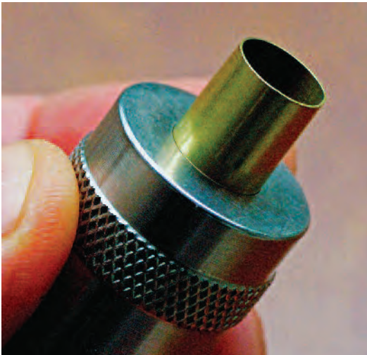
As part of checking crimp, begin by inserting the cartridge casing into the case gage backward, to ensure its rim will fit completely into the gage.
