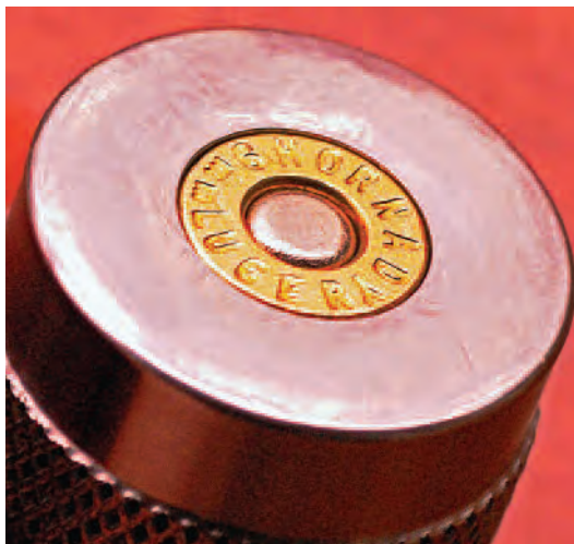
When excess case flare has been removed, the round should drop fully into the case gage.
