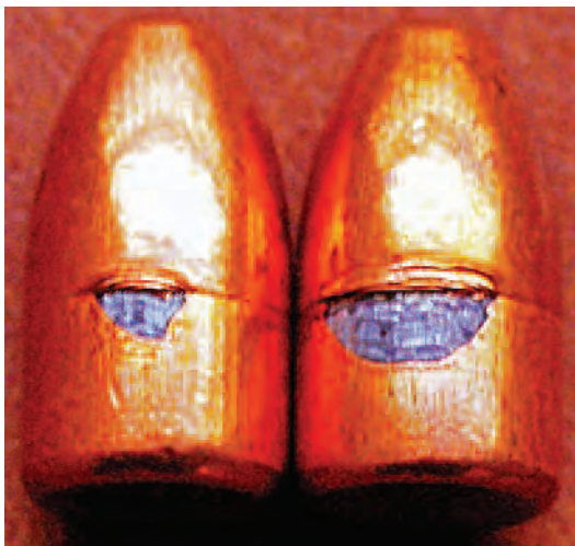
Insufficient flare will lead to the sharp case mouth cutting through thin plating.
