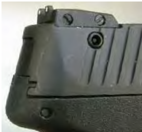
The rear sight is screw-adjustable for windage and elevation. Just below it on the right side is the Taurus key-lock for storage.
