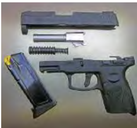
Takedown for cleaning is simple and easy. Five parts.
