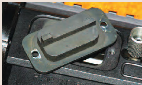
The ejection port cover contains the ejector. Switching the plate to the other side of the rifle changes its ejection pattern.
