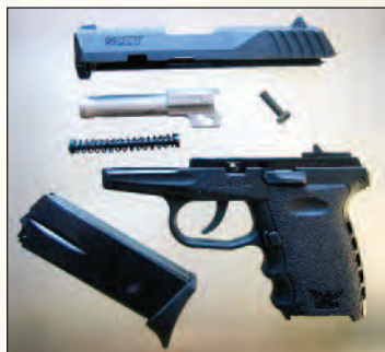
Above: Right side of the SCCY CPX-2. Right: Takedown and reassembly are easy. The captive recoil spring is a nice touch.
