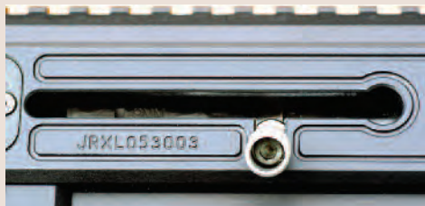
The bolt may be manually locked to the rear by aligning the bolt handle with the vertical leg of the "T" then rotating it down.
