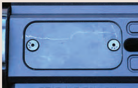
On the left side, a steel plate covers a second ejection port.
