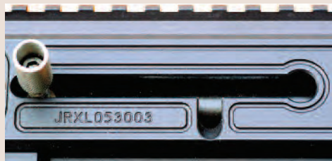
The bolt reciprocates in a T-shaped track.
