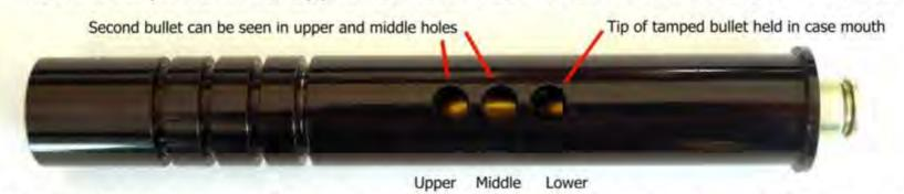
The bullet tip appears fully in the lower hole array, but the base of the second bullet above does not... therefore, this indicates that the steel balls should be positioned in the lower array of holes when reloading this length of bullet.
