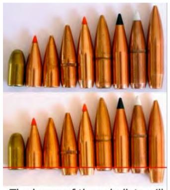
The bases of these bullets will tamp into an expanded case mouth to approximately the red line shown above.
