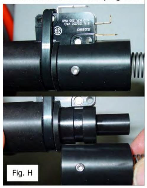
The setscrew is present to secure the cap to the top of the switch section. All that is required is that the setscrew enters the machined groove on the switch section. It will prevent the cap from coming off. Do not tighten the setscrew or you might distort the bore of the switch section and cause bullets to jam.
