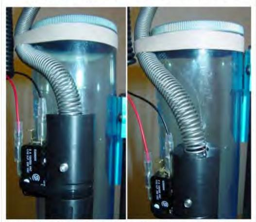
A wide rubber band may be used to help support the output tube spring and at the same time, provide an acceptable amount of slack in the tube. The rubber band shown is a #84 purchased at Staples. It's 1/2" thick and approximately the same diameter as the powder reservoir). These images show a 223 dropper mounted to a Dillon RL-1050 press (as viewed from standing in front of the press).
