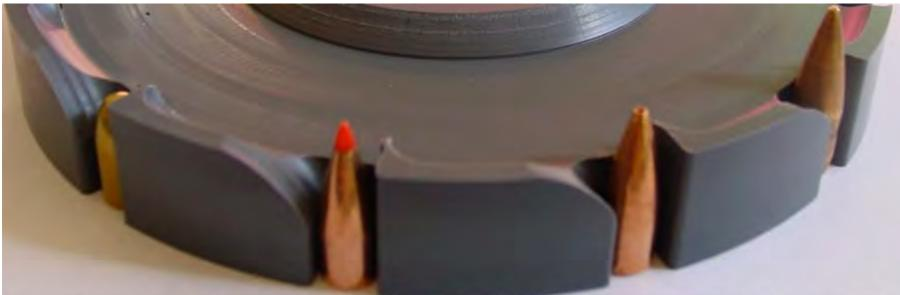
For shorter bullets, only use the upper section of the collator plate. If you also use the spacer, bullets can become stacked in the collator plate slots and cause mis-feeds and jams.
