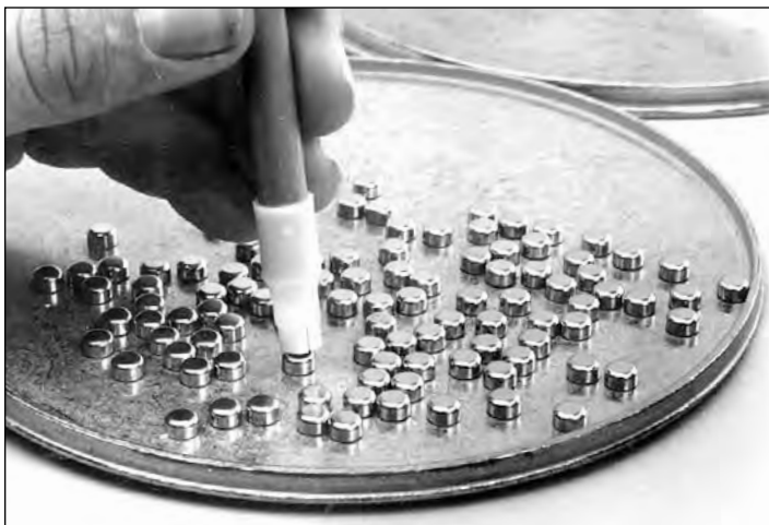
Fig. 13: All of the primers must be shiny side up.
