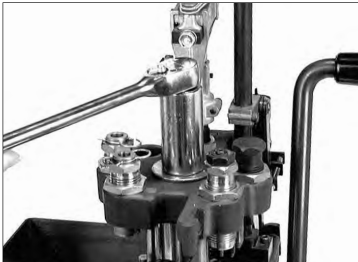
Fig. 21: Use a 15/16" socket wrench to remove the toolhead bolt.
