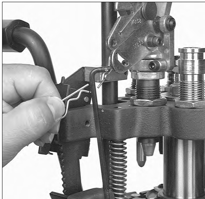
Fig. 20: After removing the clip and disconnecting the rod, replace the clip in the rod for safe-keeping.
