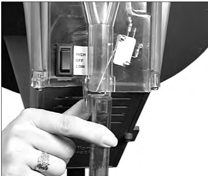
Fig. 5: The end of the casefeed tube marked "up" snaps into the clip at the base of the casefeeder motor housing.
