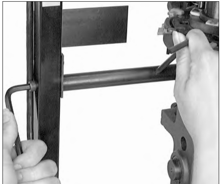
Fig. 3: Place an Allen wrench into the cross hole and use it for leverage to tighten the casefeed post studs.
