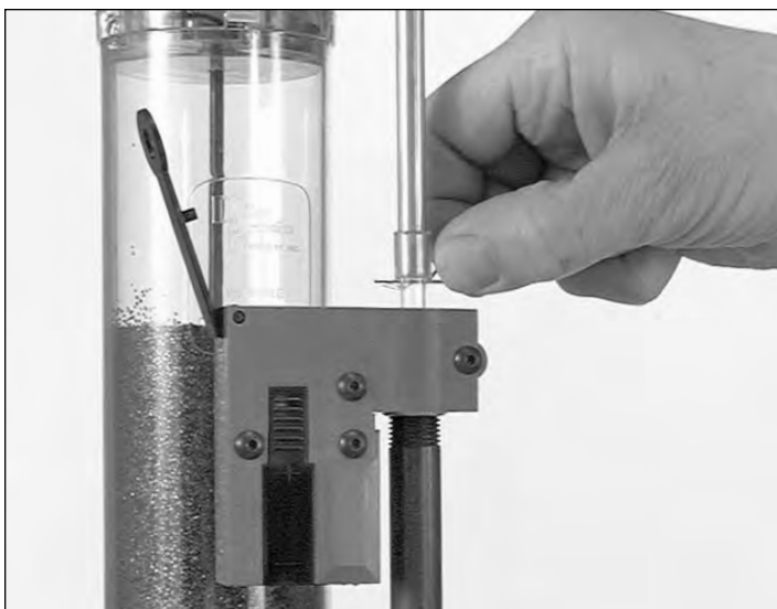
Fig. 14: When installing primers into the primer magazine, be sure the pick-up tube centers itself before pulling the clip.
