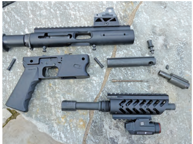
Below: Takedown requires no tools other than a pointy thing to get the pins started on their way out. Field stripped, you see the bolt head, and the barrel/jacket and magazine-well/pistol grip assemblies. These three components are the ones switched out to change calibers. The bolt carrier and tubular receiver assembly works with all calibers.
