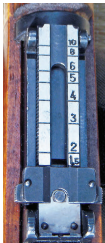
Top view of the M39 rear sight set up as a tangent sight.
