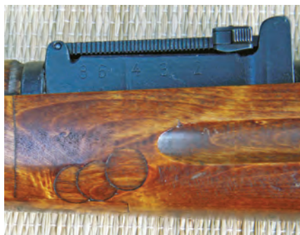
Side view of M39 rear sight showing the finetuning increments between range scale numbers. Note also the factory repair of flaw in the wood via three hardwood dowel plugs.
