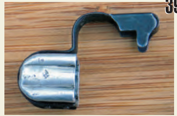
K31 muzzle cap for protection of the muzzle crown and front sight, as well as prevention of bore obstructions during rough maneuvers on snow-covered, mountainous terrain. Note Swiss Cross embossed on side.
