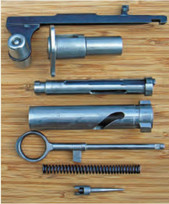
K31 bolt components (top to bottom): bolt handle, bolt cap, bolt cylinder with extractor installed, bolt body (note spiral cam slot), cocking piece, mainspring and firing pin.
