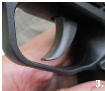
Photo 1: The controls: Takedown latch, slide latch, and magazine release. Photo 2: Simple design prevents problems. The sear and disconnecter are shown. Photo 3: A beautiful trigger. No “flipper” safety, no ridges, wide and smooth. Photo 4: A small opening at the rear edge of the barrel lets you see a chambered round. Photo 5: The magazine with the extension accommodates all three fingers.
