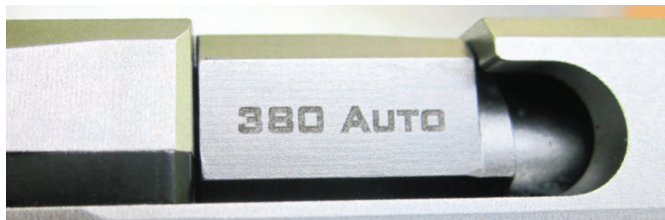
Above: The SCCY CPX-3, field-stripped. Takedown is easy. Left: On the right side of the slide, a really neat design touch. The ejection port is extended forward, so live rounds can be easily removed.
