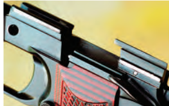
The slide rails in the frame, to either side of the mag well, have been removed to decrease friction during cycling.
