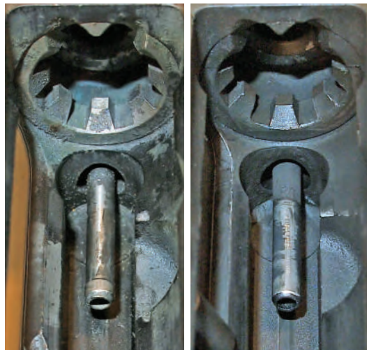
Above Left: A proper gas tube flare for sealing against the gas key on the bolt carrier group.
