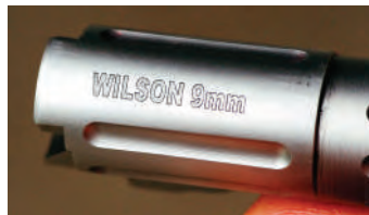
The top of the EDC X9's "low friction barrel" has no locking lugs.
