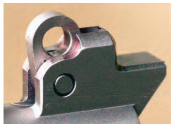
The design does retain the 1911's traditional swinging link.
