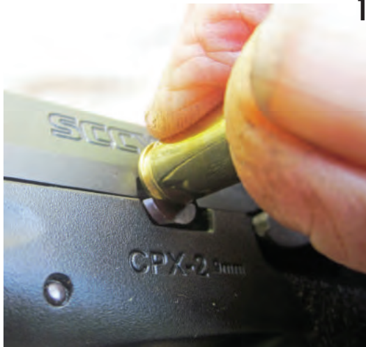
A cartridge rim is the perfect tool for removal of the takedown pin.
