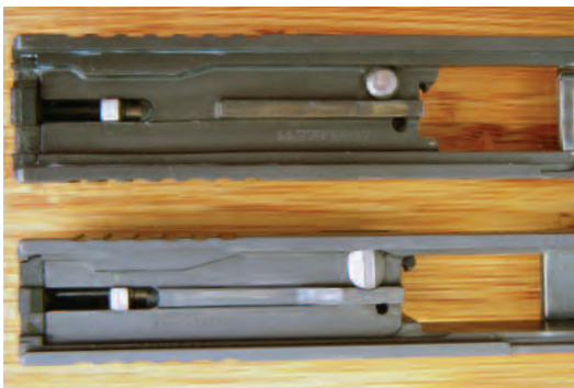
G26 slide (above) compared with G43 slide (below). Note the narrower width of the G43 slide as well as the modified shape of the G43 firing pin safety.
