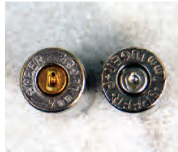
The primer of the fired case on the left exhibits the characteristic firing pin indentation surrounded by a raised rectangular area made by GLOCK pistols with conventional strikers. The case on the right was fired from a G43 with the new striker design.
