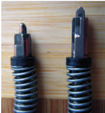
The newer configuration of the GLOCK 43 striker (left) contrasts sharply with the older style GLOCK striker (right) in this case from a G26.
