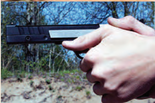
This is NOT the gun for every hand. The slide rides so low that the slide will rub fleshy hands raw after a few dozen shots. Depending on what stocks (grips) you have on the gun, and how you grip the pistol, your thumbs may rub the slide.
