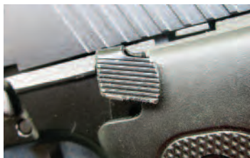
Above: A single ambidextrous lever operates the slide release and lowers the hammer. Below: The pistol, ammo box, target.
