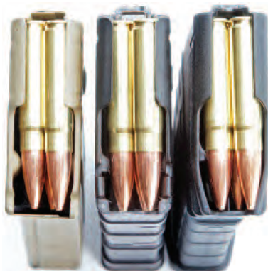
From left, a G.I. style magazine, a Lancer and a MagPul P-Mag. Note the difference in size of the guide ribs and where the ogives touch.
