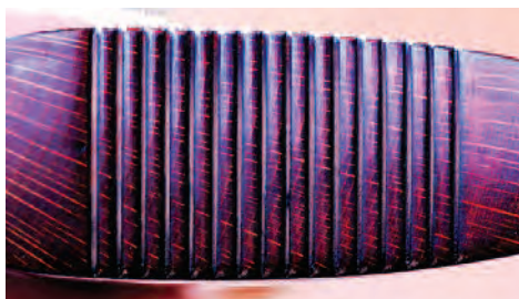
The crescent butt has no buttplate, but instead has serrations cut directly into the wood.
