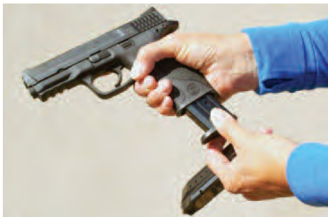
Figure 4 – The magazine release button is pressed and, with the thumb and forefinger of the non-firing hand, the partially spent magazine is removed from the gun.
