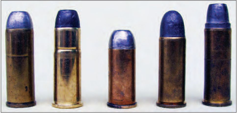
Figure 2: The stumpy and underpowered .44 Russian round (center) compared with its more effective black powder contemporaries the .44-40 (immediate left) and the .45 Colt (far left). The two smokeless rounds later descended from the .44 Russian are the .44 Special (near right) and .44 Magnum (far right).
