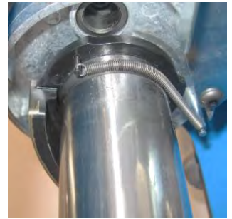
Reinstall Index Ring Spring
