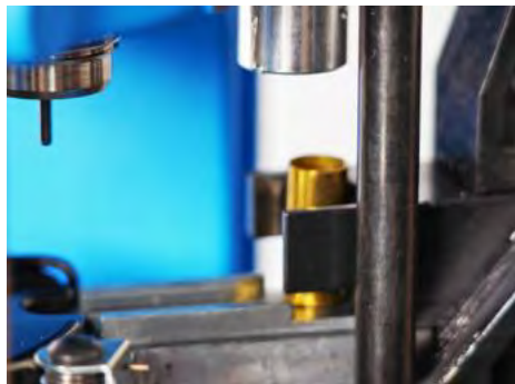
Station 1-Case dropped onto Station 1 Locator
