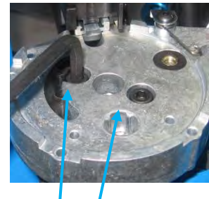
Remove Platform Mounting Screws and the Platform
