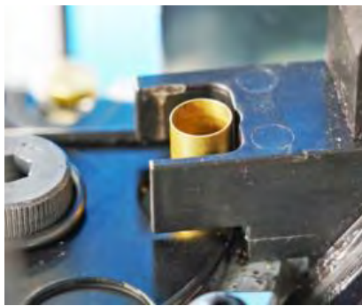
Station 1 Station 1-Case Inserted into Shellplate—full aft stroke
