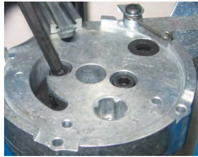
Loosely tighten Mounting Screws
