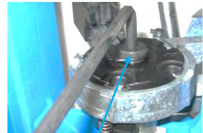
Remove Bolt and replace Shellplate
