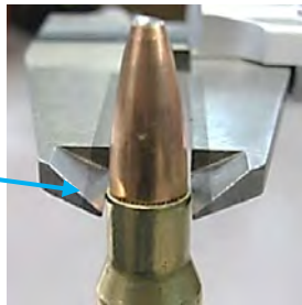
Crimp –reduce diameter no more than .001-.002”
