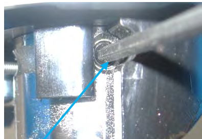
Loosen Brass Tipped Locking Set Screw with an Allen wrench
