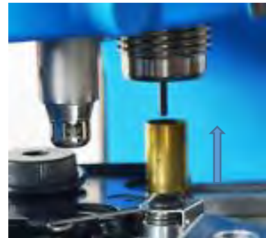
Station 1-Case Inserted into Size De-prime Die—down stroke
