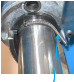
Carefully remove Indexer Return Spring from the two pins
