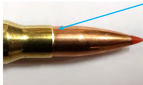
Excessive crimp may show up as a “bright ring” at the top edge of the case neck
