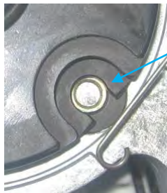
Primer Punch and Cup Centered in Shellplate
