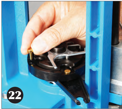
22 You may now place the three brass Locator Buttons (from the RL 550B Caliber Conversion Box) into the remaining holes in the Platform. Their proper positions are shown at right in photo 23.
