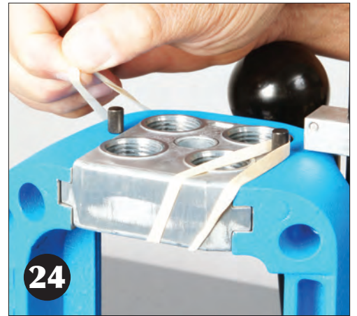
24 The rubber band intended to keep the Toolhead Pins in place during shipping may now be removed in preparation for installing the Automatic Powder System.
