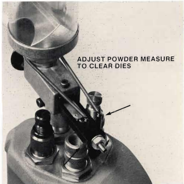
Figure 9: Top view of press with powder bar pushed in
