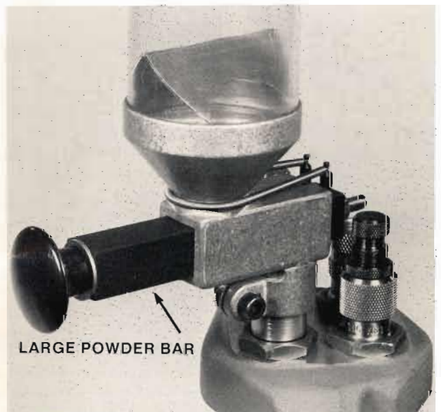
Figure 7: Close-up picture of Powder Measure with large powder measure bar
