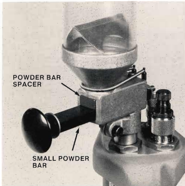
Figure 8: Close-up picture of powder measure with small bar and spacer
