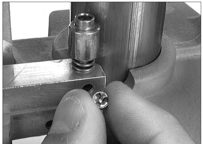
Figure 34 – Placing a primer in the primer cup at Station #1.
