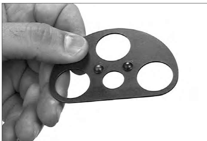
Figure 6 – Locator “dimples” on the AT 500 shellplate cover.
