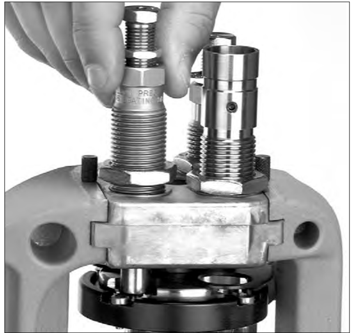
Figure 17 – Installing the bullet seating die in Station #3.
