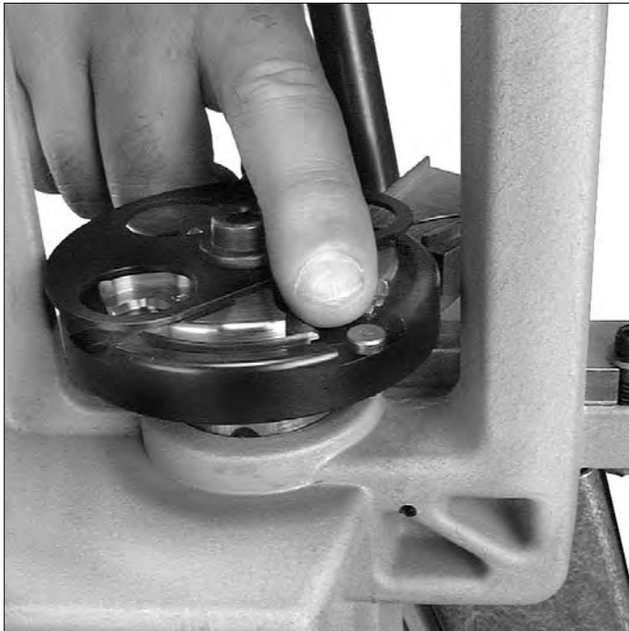
Figure 32 – Installing a brass locator button in Station #2.
