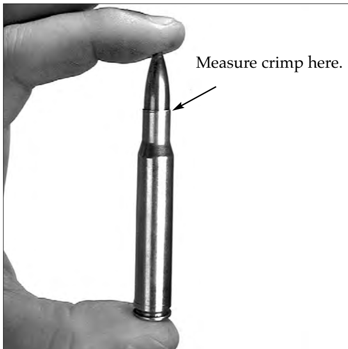
Figure 20 – A properly crimped rifle cartridge.
