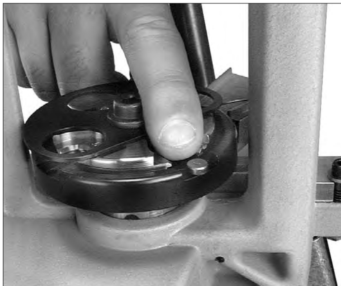
Figure 21 – Installing a brass locator button at Station #2.
