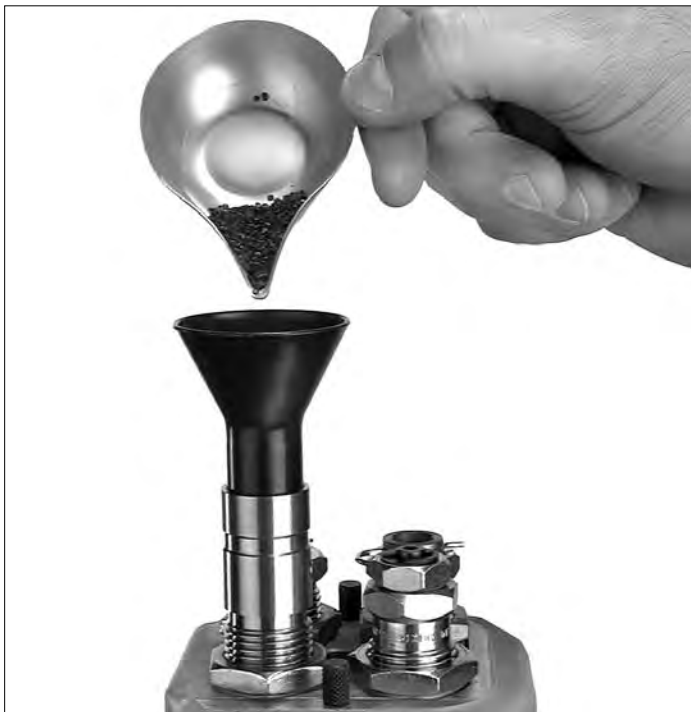
Figure 35 – Charging the case with powder at Station #2.
