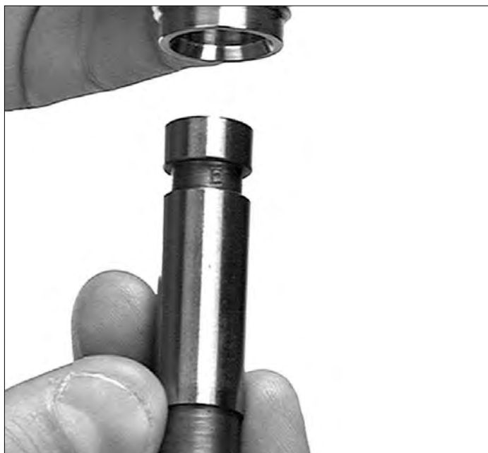
Figure 26 – The groove in the pistol powder funnel.
