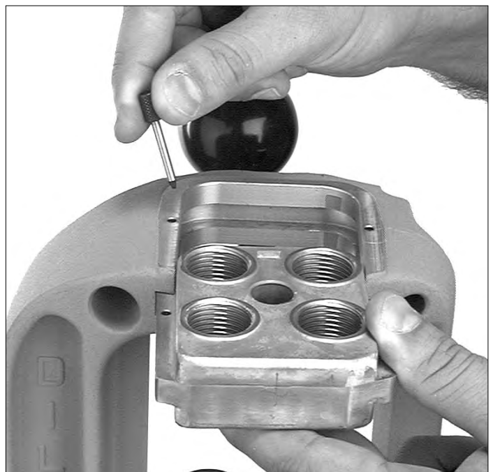
Figure 10 – Removing the toolhead.
