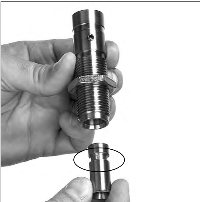
Figure 16 – The groove in the rifle powder funnel.
