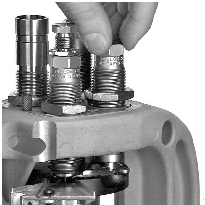
Figure 19 – Installing a taper crimp die in Station #4.
