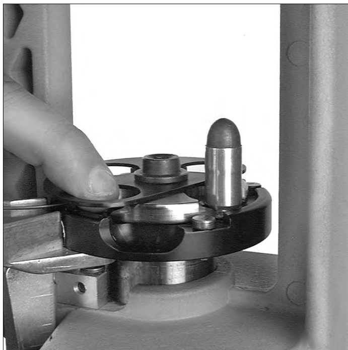
Figure 37 – Advancing the shellplate to Station #4.
