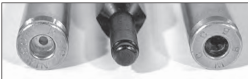
Photo "B": The case on the left shows a properly swaged primer pocket.
