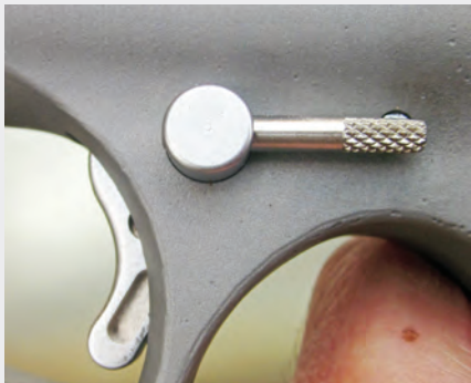
The latch for the barrel unit.
