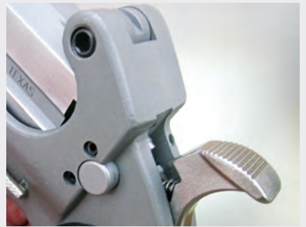
The hammer-block safety, shown on-safe.
