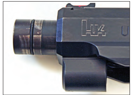
The rubber “O” ring is an ingenious way of ensuring more consistent lock-up between barrel and slide.
