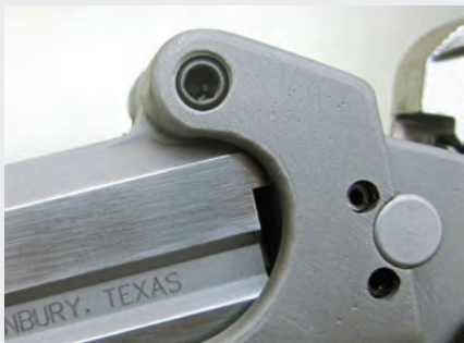
The barrel hinge is much sturdier than the one on the old Remington.
