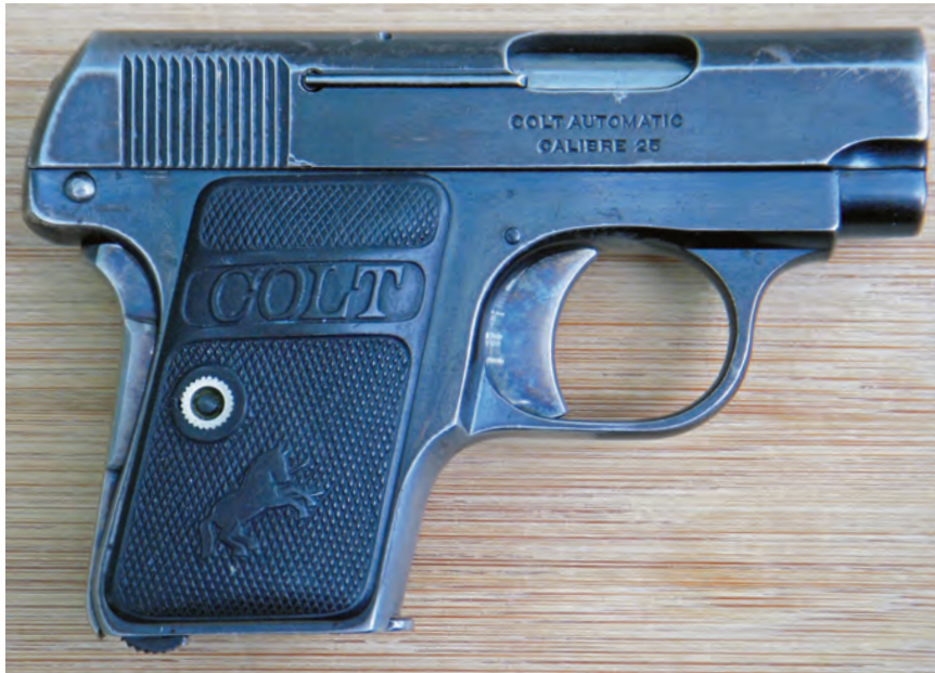
Author's blued, Colt Model 1908 Vest Pocket pistol, caliber .25 ACP with molded hard rubber-stocks and color case hardened trigger and grip safety. Note Colt's signature symbol, the "Rampant Colt" on the stock panel. This gun was built in 1920.
