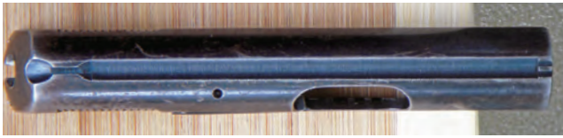
Top view of the slide of author's Colt M1908 Vest Pocket .25 ACP pistol showing the tiny front and rear sights milled into it. Note also the pronounced machined channel, which acts as a "guttersnipe" sighting system for fast work at close range.
