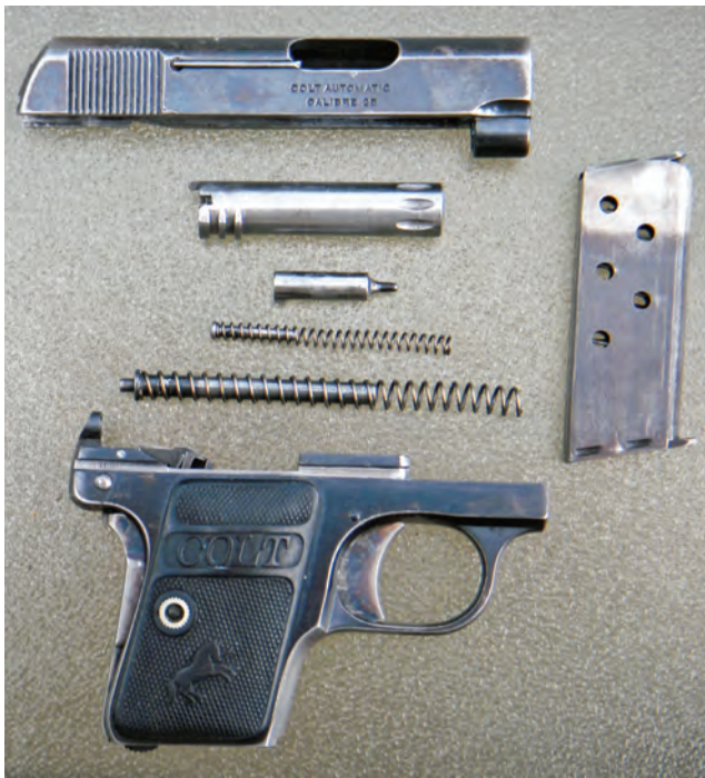
Author's Colt M1908 Vest Pocket .25 ACP pistol field stripped. From top to bottom: Slide, barrel, firing pin, firing pin spring with firing pin spring guide, recoil spring with recoil spring guide, and the frame. To the right is the magazine. Note the small, cylinder-shaped projection sticking out of the rear flange of the recoil spring guide for engaging the Tansley magazine safety device when the mag is removed.
