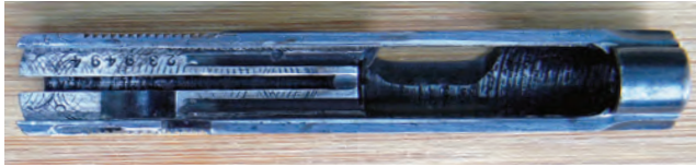
Looking at the underside of the slide from the author's pistol, one can see the guide slot milled through the 6 O'clock portion of the firing pin channel and through which the firing pin's cocking stud travels. The milled out area below the firing pin channel, commencing about one-half inch from the back of the slide is part of a safety feature which allows the connector to engage the sear only when the slide is fully forward and which prevents the weapon from firing out of battery.
