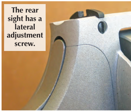
Double-Action-Only, no hammer spur to snag on the draw.
