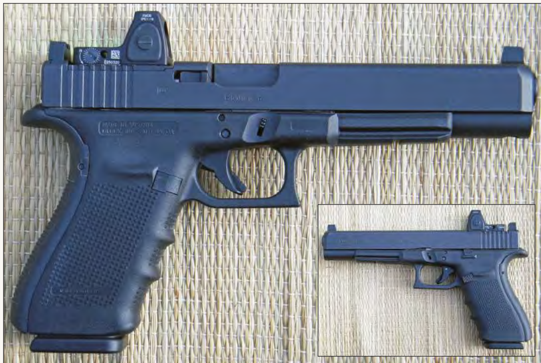
The author's GLOCK G40 10mm pistol shown here with Trijicon® Adjustable LED RMR reflex sight, Trijicon suppressor-height tritium sights, and medium-reach beavertail backstrap extension. Note the Trijicon-supplied adapter plate sandwiched between the mounting base and the sight base.
