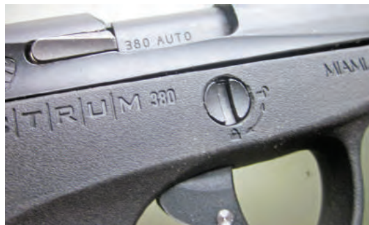
Takedown latch, above the trigger. With the latch slot turned to horizontal, slide unit is moved off toward the front.
