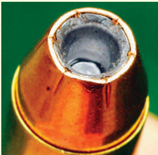
The short overall length and gaping hollowpoint of the Super Vel 90-grain JHP +P might seem it would lead to feeding failures, but, at least in the five guns with which Thomas tested it, that proved to not be the case.
