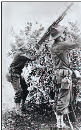
American Doughboys with a French Model 1914 Hotchkiss machine gun on a camouflaged anti-aircraft mount. A posed 1917 training photograph, note the empty loading gate and absence of ammunition "sticks." National Archives photo.
