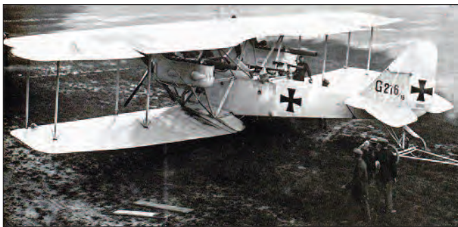
An AEG Grosskampfflugzeug (“heavy bomber”) Mark V at a German aerodrome in 1918. Note the twin, rear-facing machine guns on separate mounts just aft of the upper wing. This was the kind of twin-engined bomber shot down by Lt. Colonel William T. Dillon from the ground with a model 1914 French Hotchkiss 25-shot machine gun. Internet photo.
