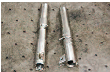
Here we have nearly completed 1911 barrel and barrel bushing sets.
