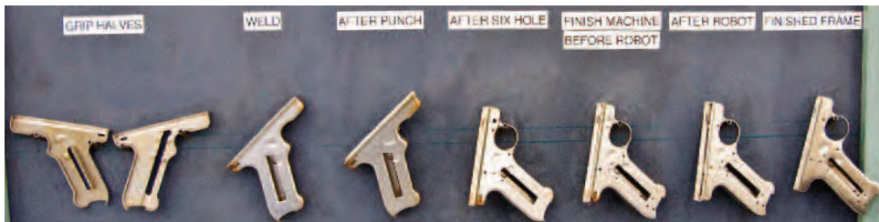
Here you see the various stages of a frame being made for a Mark III stainless .22 pistol. At each stage, the dimensions are extremely critical; automated machines are exactly controlled by computers.
