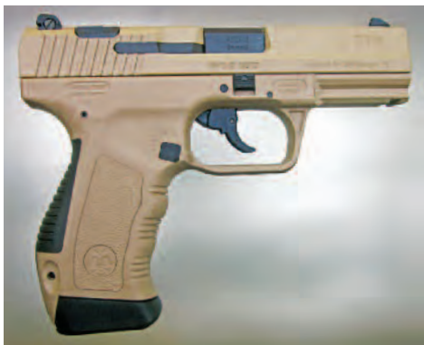
Push down on the decocker forward of the rear sight and the striker is un-cocked.
