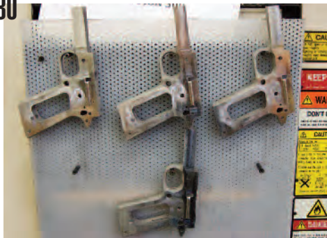
These are aluminum 1911 frames in various stages of completion at a drilling station.
