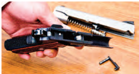
Ruger's aluminum-framed 1911 features a titanium feed ramp to resist damage from feeding hollowpoint ammo.
