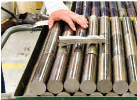
Shown on top of a cart of stainless steel bar stock is a nearly finished 1911 slide made from one of those bars.
