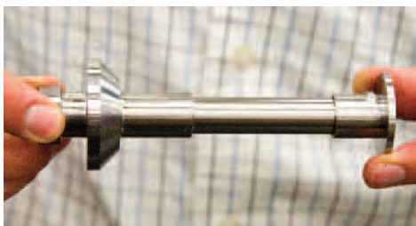
This is a semi-finished stainless 1911 barrel and barrel bushing set. These parts are manufactured together, and remain as a mated pair until final assembly.
