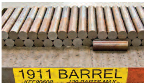
Here is raw bar stock waiting to be transformed into 1911 barrels and barrel bushings.
