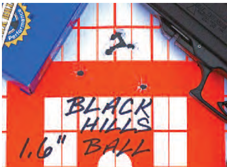
Black Hills "blue box" hardball reloads put five rounds into this respectable group at 50 feet from the bench, but POI was 3-1/2" above POA with the adjustable rear sight bottomed out.
