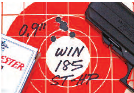
Winchester 185-gr. Silvertips put five rounds into less than an inch. POI was 1-1/2" above POA.
