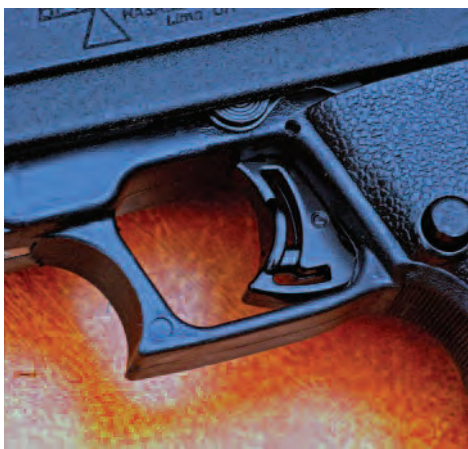
The trigger is plastic. Trigger pulls were quite smooth, if a bit long. The trigger broke at five pounds even.
