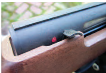
The Mitchell PPSH 41/22's safety lever, shown here in fire position.
