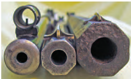
Figure 3: The “business end” of the 1870 .50-70 Remington Rolling Block, at right, compared with a .30 caliber Model 94 Winchester at center, and a .22 caliber Model 43 Mossberg bull-barrelled .22LR Target Rifle at far left. The old buffalo gun had a hard life, to judge by the battering on its muzzle.
