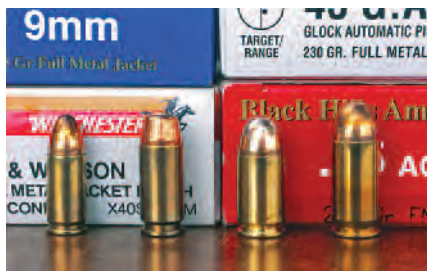
The goal with .45 GAP was to produce a .45 caliber cartridge about the same overall length as 9mm or .40 S&W, and considerably shorter than .45 ACP. As this layout shows, the attempt was successful.
