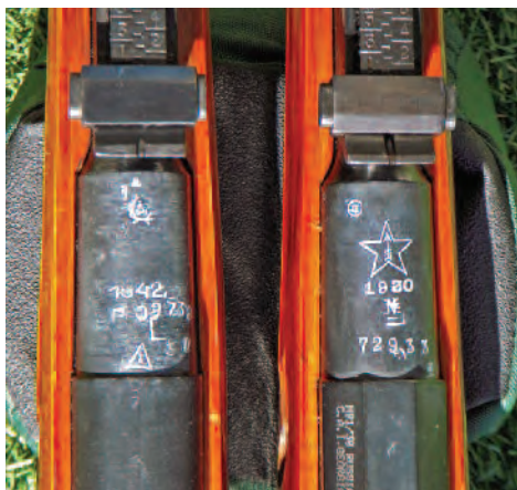
On the left is the top view of the receiver and barrel chamber area of author's Izhevsk round receiver 91/30 Mosin-Nagant. Note circumferential tool marks on the barrel and longitudinal ones on the receiver as well as less than stellar execution of arsenal markings and characters on barrel, which are consistent with wartime expediency measures. The author's prewar Tula hex receiver 91/30 exhibits a much better finish and more crisply applied markings and characters.
