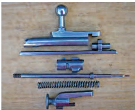
Disassembled 91/30 Mosin-Nagant bolt components from top to bottom: bolt body; bolt connector; bolt head, note the substantial twin forward locking lugs and how the extractor resides in its dovetail; firing pin (striker); firing pin spring; and cocking piece.
