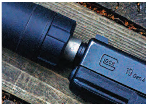
The rear of the silencer unscrews to allow piston replacement. By pulling it forward and turning it to the next internal notch, the end user can adjust point of impact to more closely match POA of the unsilenced pistol.
