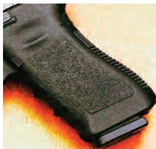
Note the author has cut a piece of ladder tape to follow the contours of the lozenge of cobblestone roughening already existent on the Glock grip.
