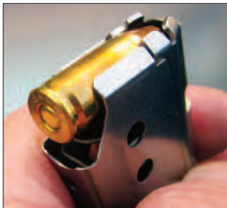
The top of the Boberg XR9-S pistol's rearward-feed magazine with a round in place.
