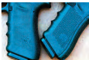
(From Left) Left Side Panel: The left grip panel receives a piece of ladder tape. Note the pieces of skateboard tape on the backstrap. RFT-2 and RTF-4: Two attempts by Glock to factory roughen their grip frames have been the RTF-2 and the RTF-4 (the latter being standard issue on Gen-4 Glocks). Still the author prefers grip tape to either factory treatment.
