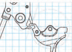
Patented Ruger® Friction Reducing Cam
