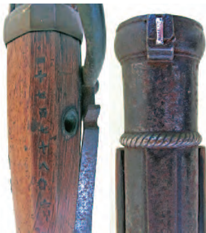
Figure 2 (Left): Detail of the upper grip, with Japanese inscription translating to a converted western date of 1680. Note also the brass-lined tunnel for the slow match to right of characters, relaxed spring and hammer at right. Right: Detail of the Dillon matchlock muzzle, showing its slight “belling,” the “high visibility” silver front sight, and brass “rope” applique that terminates the fore-piece below and the raised barrel rib above.
